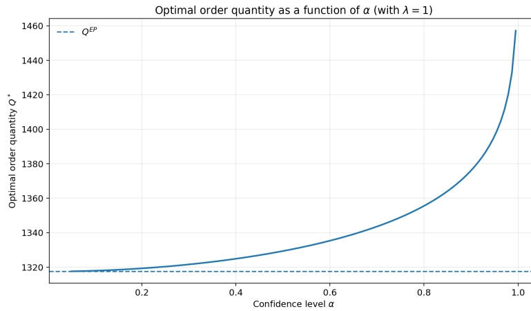
Figure 4.8: Optimal order quantity Q^* as a function of the confidence level \alpha , using \lambda = 1 .
